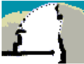
Figure 3: Occupancy Map Used for Exploration “Obstacle” cells are black, “clear” cells are white, “unknown” cells are grey. Frontier cells are marked by small circles.
